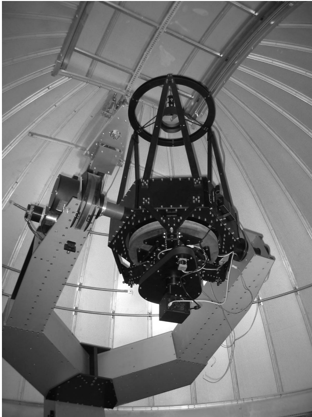
Fig. 1. Torus Precision Optics (now Optical Mechanics, Inc.) CC05 telescope at the University of the Virgin Islands. Note the long equatorial fork allowing observations to the horizon at 18° North latitude. Also visible are the 12-position filter wheel and the Finger Lakes Instruments CCD camera. A single serial cable from the control room controls the entire observatory system. A second USB cable controls the camera. Optical encoders on the RA and Dec axes provide 0.1" precision. Secondary focus, filter position, and dome position are "open-loop" control systems driven by extremely reliable servo motors.
